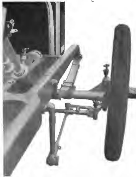
STEERING CONNECTIONS OF FOUR-CYLINDER OLDS TOURING CAR.
